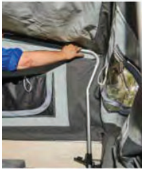
Use the Velcro to attach the roof bow to the roof
