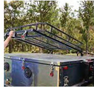
Push the rack upward towards the opposite side of the camper
