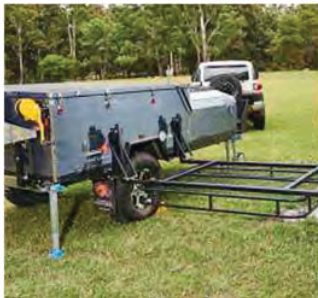
The rack can now be locked in this down position using the pins from the locking latches
