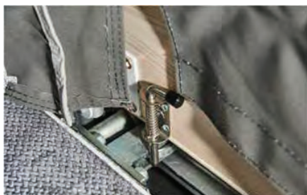
The locking pin needs to be released inside before sliding the bed out
