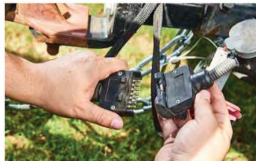
Step 4 - Disconnect all electrical plugs
