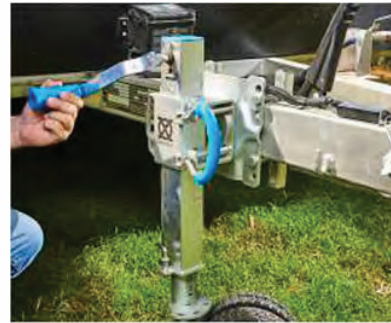
Step 2 - Lower the jockey wheel to take the weight of the trailer
