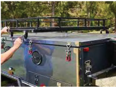
Release locking latches on the utility rack
