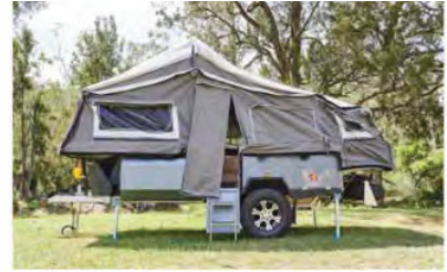
Here's what it should look like with the bed (centre) bow raised
