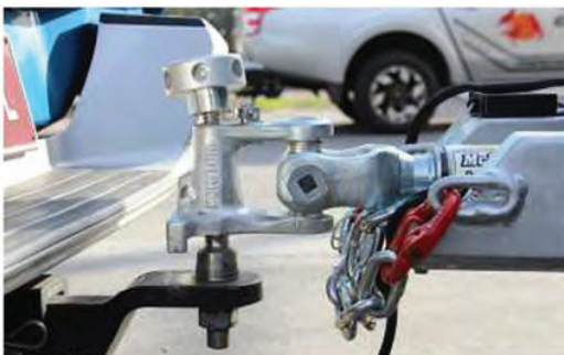
Step 7 - Carefully pull away from the trailer with the tow vehicle until the coupler is disconnected.
