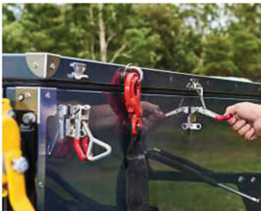
Release the over-centre catches
