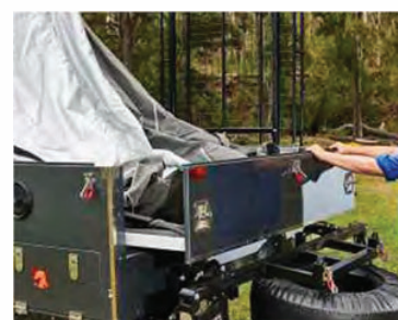
After unlatching the rear pin slide out the bed section until fully extended
