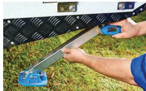
Step 8 - Lower stabilizer jacks and adjust them using the supplied jack wrench until they begin to get snug with the ground.
