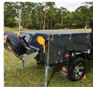
Carefully lower it down making sure it clears the rear slide out of the camper
