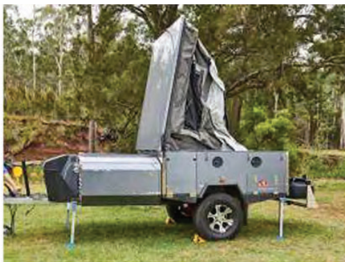
Use the front winch to get the lid past 90 degrees
