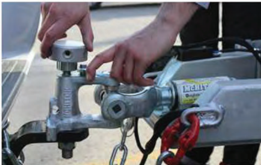
Step 3 - Remove locking pin and lift automatic locking lever on the McHitch
